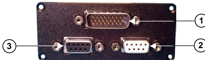
Figure 7 – Connector Panel for Profibus Models
