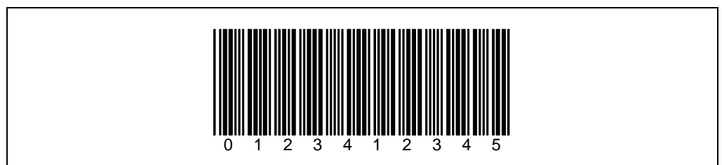
Fig. 6-1: Bar code pattern (Code 39; module width 0.35 mm; Print ratio 2:1)
