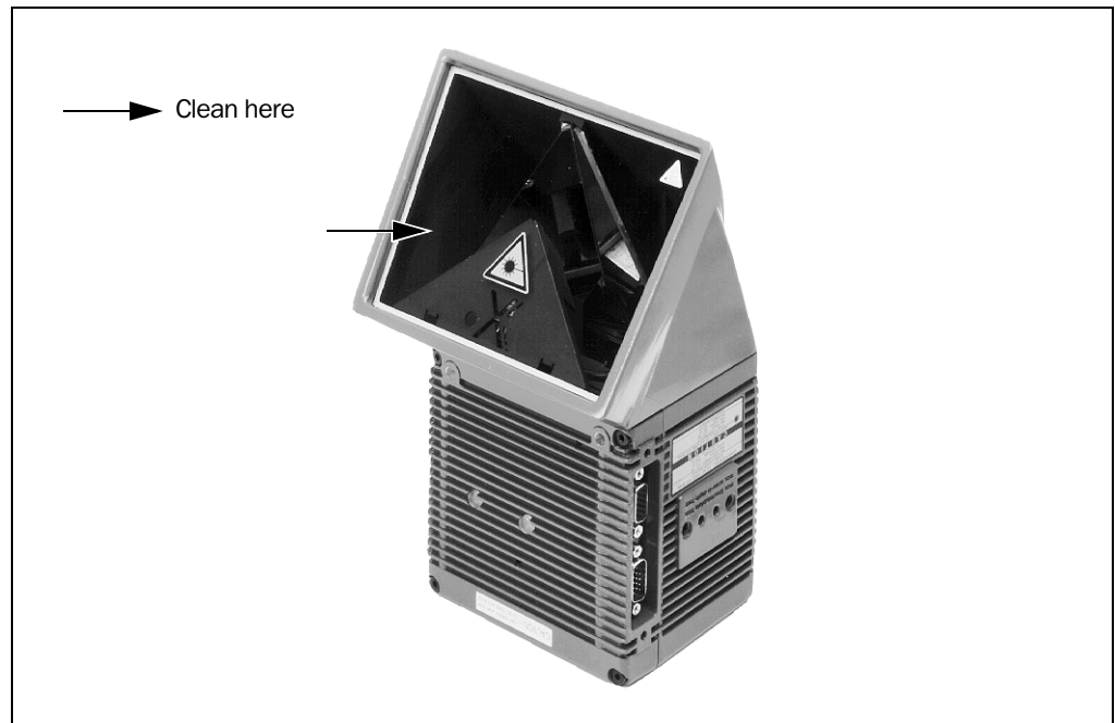
Fig. 7-1: Cleaning the reading window
