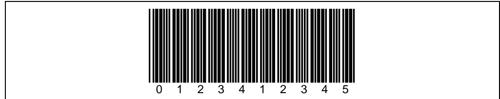
Fig. 6-1: Bar code pattern (Code 39; module width 0.35 mm (13.8 mil); Print ratio 2:1)
