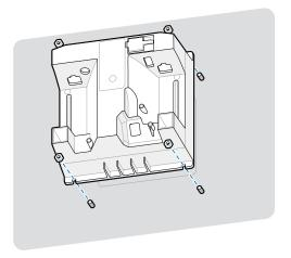
There should be clearance in the housing for most M4 sockets. In some cases, an open-ended wrench may fit better.
